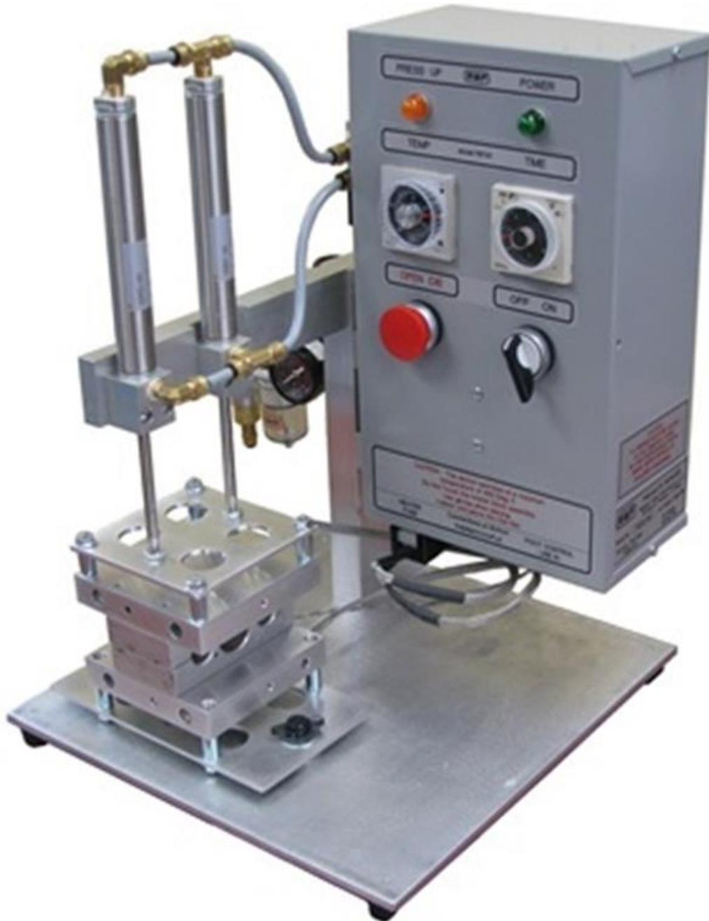
The PBX Models are benchtop units consisting of a pneumatic vertical press controlled by dual air cylinders and activated by use of a foot pedal thus allowing for hands-free (2-hand) positioning of rubber cord stock.
