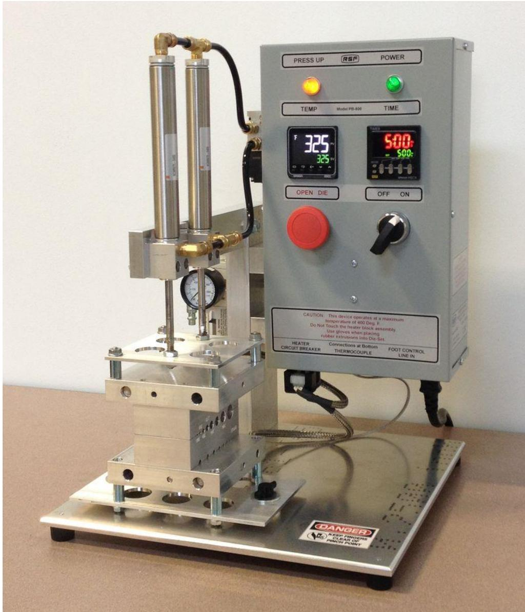
The PBX Models are benchtop units consisting of a pneumatic vertical press controlled by dual air cylinders and activated by use of a foot pedal thus allowing for hands-free (2-hand) positioning of rubber cord stock.
